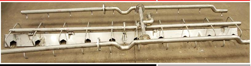
Sand Jetting systems remove solids that have been deposited in the bottom of a separator. They fluidizes the solids by use of pressurized water introduced through spray nozzles and remove the slurry through drain nozzles in the bottom of the separator. During cleaning there is no need to depressurize the separator or even stop production.
