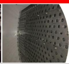
Calming Baffles are internals used in horizontal vessels for various reasons. These baffles are perforated plates with net open areas of 10%, 20%, 30%, or 50% with various hole sizes ranging from  $\frac{1}{2}$ " to larger. The baffles usually cover the liquid flow cross sectional area of horizontal 2-phase and 3-phase separators and can be designed to extend in the vapor flow area of 3-phase separators to minimize the vapor maldistribution.
