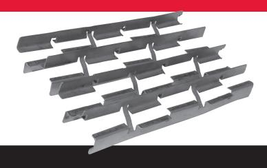
AMACS Structured Grid Packing (ASGP) is a good choice for applications that have fouling, erosion, coking and process upset tendencies. ASGP is extremely structurally durable and has a high void space percent suiting it well for turbulent vapor streams in the 1000° F (538°C) range.
