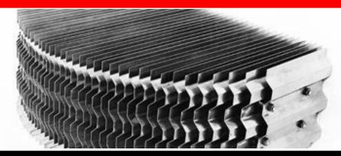
Vanes are parallel corrugated sheets held at fixed distances which creates a serpentine flow path for mist laden gas. As the mist laden gas flows through the vane, it changes direction several times subsequently resulting in the introduction of a certain level of centrifugal forces to fluids. Inertia carries the heavier liquid droplets onto the vane surface, where they adhere and coalesce to form a liquid film which trickles down due to gravity.
