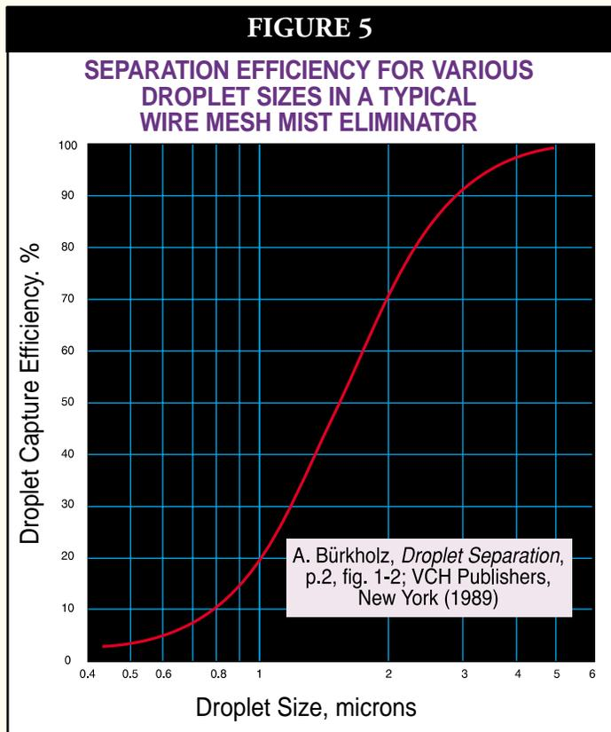
Droplets  $\sim 20 \mu\text{m}$  and greater are primarily collected by means of Inertial Impaction whereby the target is directly in the path of the streamline, as shown in Figure 4a. Figure 6 depicts a profile of the ACS PlatePak™ vane. The entrained droplets, due to their
