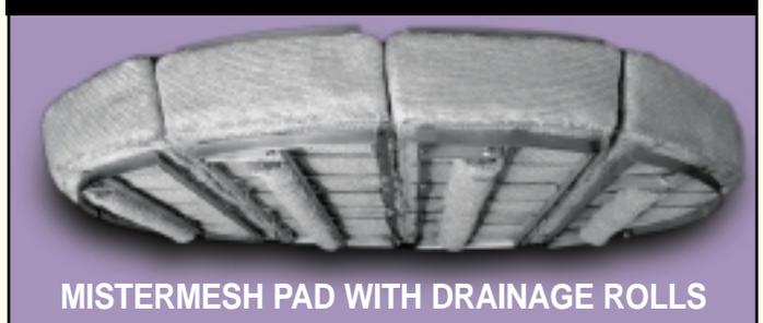
Once filled, liquid from the pad above is drawn through surface tension to the coils, thereby establishing distinct regions for liquid drainage and liquid collection in the upstream layers. Figure 18 compares the pressure drop and flooding point of both conventional and MisterMesh® Mist Eliminators.
