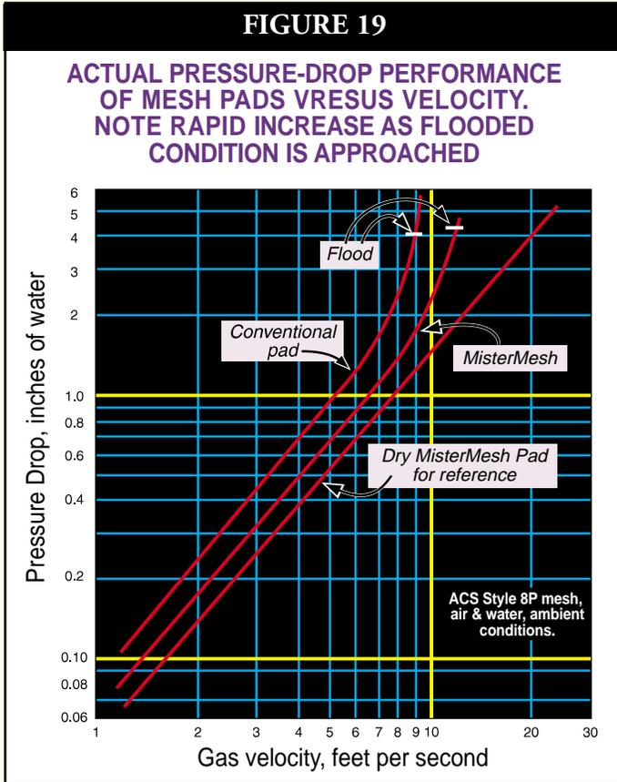
Throughout the industry there is ongoing debate as to whether the mesh should be positioned up- or downstream of the vane element. Engineers at ACS have performed exhaustive comparative testing on pilot plants and have much field data proving that the mesh is indeed affective upstream of the vane, unless the vane element is used as a pre-filter to protect a downstream mesh pad.
