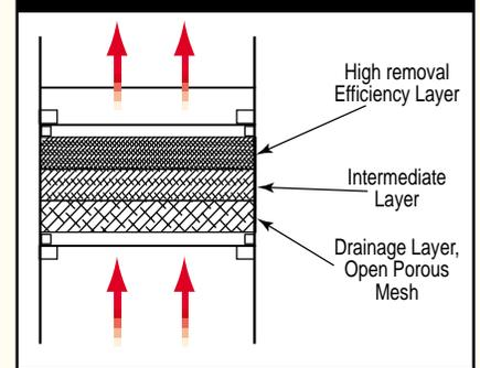
An extension of this approach is to use higher specific surface area mesh in downstream positions to enhance separation efficiency, with intermediate mesh between the collection and drainage zones. Figure 17 illustrates a Multilayer mist eliminator.
