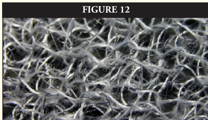
CO-KNIT MESH COALESCER THAT DEPENDS ON DIRECT INTERCEPTION
